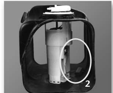
PROPERLY POSITIONED FUEL PUMP MODULE ASSEMBLY
