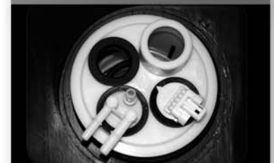
IMPROPERLY POSITIONED FUEL PUMP MODULE ASSEMBLY
