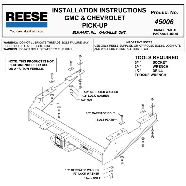
1. Remove the 12mm bolt from the bottom side of the end of the frame. Discard the bolt.
