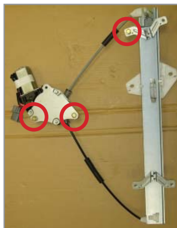
Replacement Window Regulator. Start threads on the three circled bolts.
