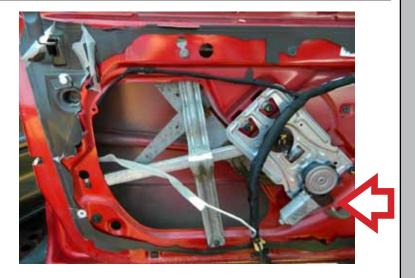
**STEP 7:** Temporarily install the power window switch to verify that the power window regulator assembly and door glass are operating properly.
