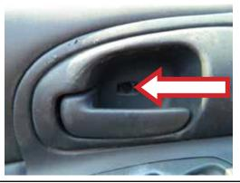
**STEP 5:** Using a pick or small flat-blade screwdriver, remove the retaining screw cover to expose the retaining screw.
