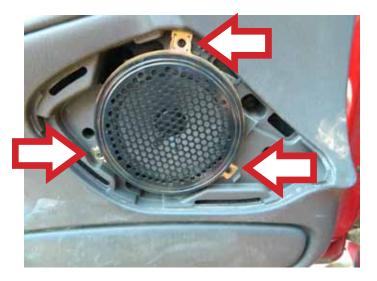
**STEP 14:** Attach the three (3) door speaker screws to the door.
