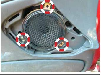
**STEP 3:** Remove the speaker from the door and disconnect the speaker. **NOTE:** To remove the connector, squeeze and slide the connector towards the door panel.
