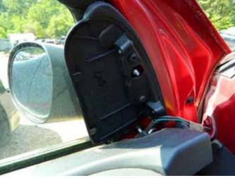
**STEP 9:** Using a trim panel removal tool, release the interior door panel retaining clips.
