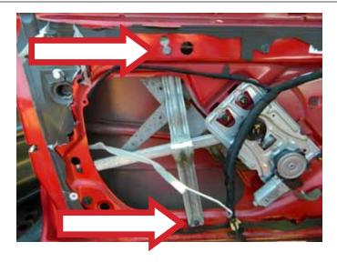
**STEP 19:** Remove the two (2) 10 mm bolts attaching the window regulator to the door glass.
