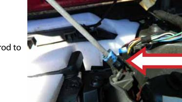
**STEP 10:** Attach the door handle latch rod to the door handle.
