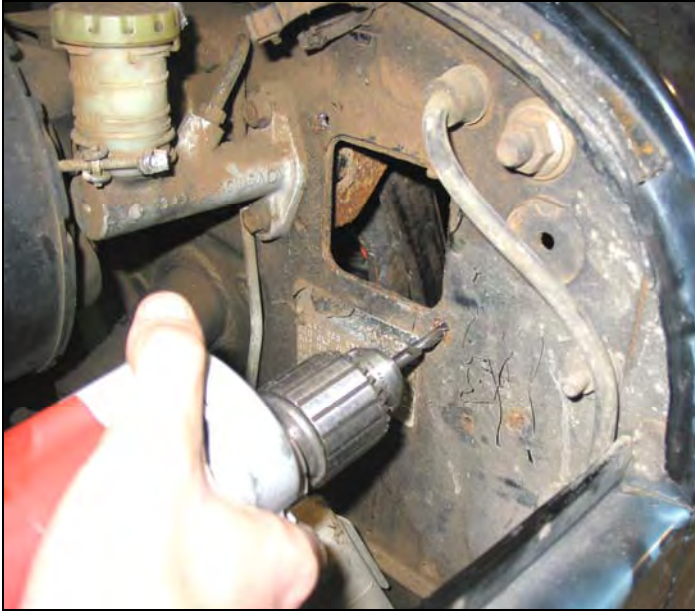
Figure 6.1.1 Fuse Block Mounting Holes
