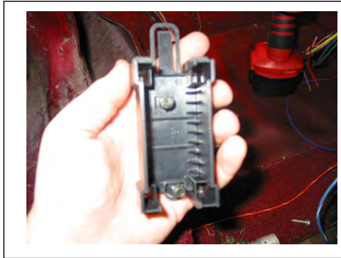
Figure 6-2 Fuse Block Base Mounting
