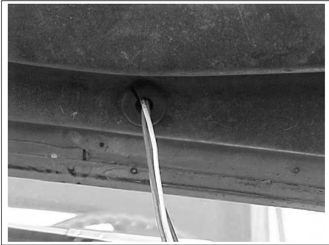
Figure 7.10 Hood Section Wiring (Routed through the bottom of the hood and grommet installed.)
