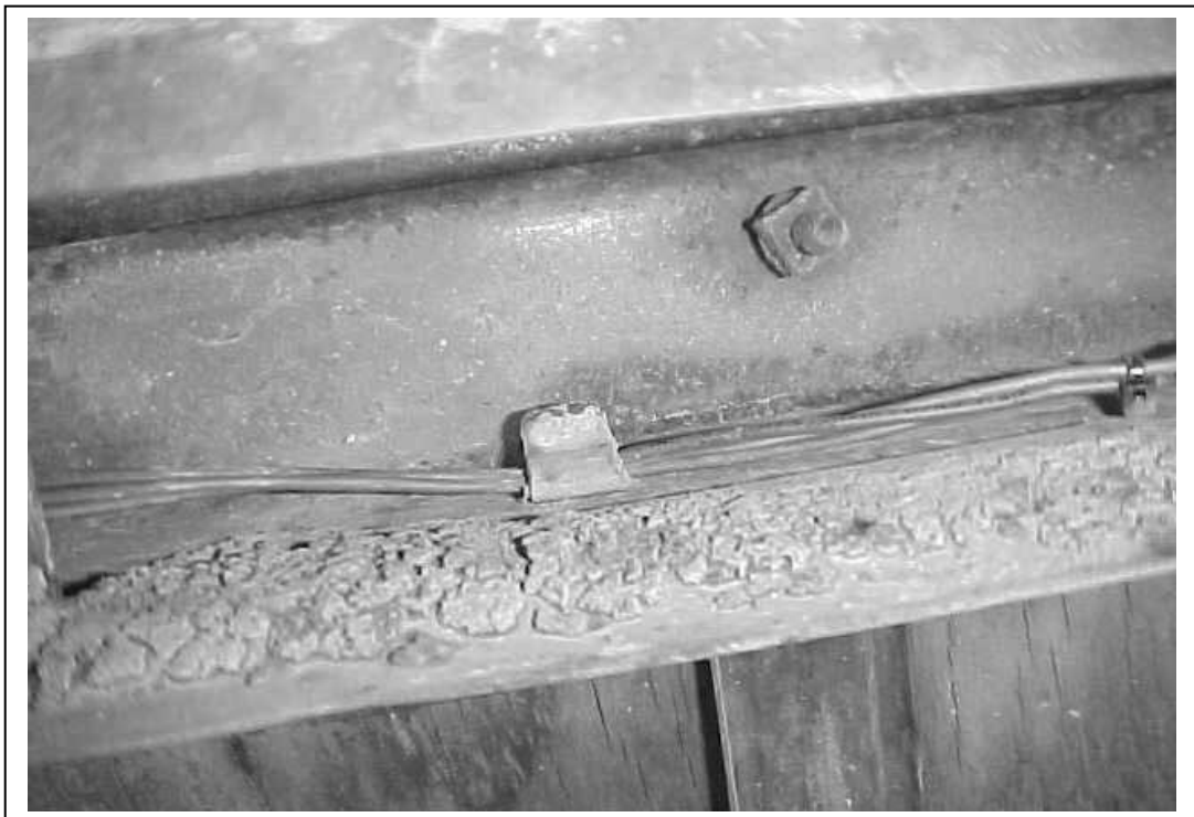
Figure 6.6 Mounting brackets are along the frame for your Tail Section mounting.
