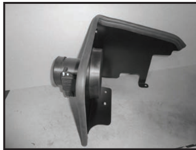
Step 12 Assemble the heat shield with the tabs placed on the outside of heat shield. Install the rubber bulb seal. Place the velocity stack adapter on the heat shield and install the MAFS placing the gasket between the heat shield and the MAFS. Once all of the holes are lined up, install the hardware and fasten securely.
