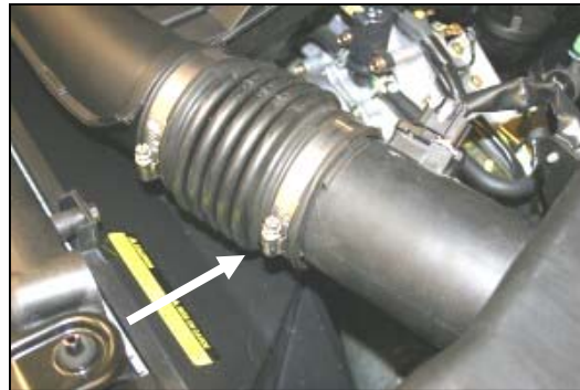
2. Loosen the hose clamp on factory airbox neck.
