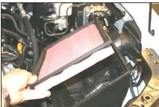
7. Remove the factory air filter.
