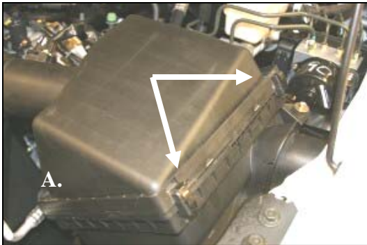
1. Disconnect negative battery cable. Unhook two latches on the factory airbox.
