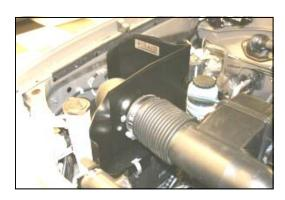
**7.** Slip MAF adapter into factory intake tube while installing CAD onto top of factory airbox. Adjust for fit, and latch 3 factory clips on factory airbox. Tighten the hose clamp on the intake tube. Replace the fan shroud bolt that was removed in step #5.
