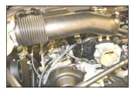
**14.** Remove the factory intake tube.
