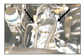
**18.** Install the vacuum tee (#12) into the 1/4"x4" hose (#13), and reconnect the factory 1/4" and 1/8" vacuum lines to the tee as shown. Install the 1/2"x13" breather hose (#8) onto the valve cover and to the MIT as shown.
