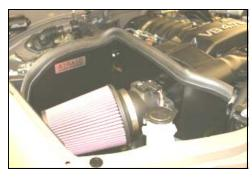
**10.** Install the Airaid Premium Filter (#1) on the MAF adapter. Next install the weather strip (#9) on the CAD as shown. Start at the front, next to the radiator, and work your way towards the back.
