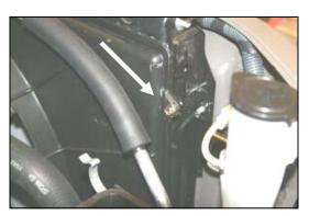
2. Loosen hose clamp where intake tube connects
