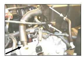
**12.** Disconnect breather hose from valve cover. Disconnect 1/8" vacuum line, and 1/4" vacuum line from the back of the factory intake tube.
