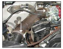
1. Disconnect the negative battery cable, then, loosen the two hose clamps on the factory intake tube.
