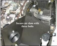
10. Position the Airaid intake assembly in place of the original, factory assembly. Using three supplied 8mm bolts and washers, mount the Airaid assembly using the three original/factory mounting points.
