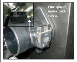
8. Using the two 8/32 Allen head screws and two plastic spacers provided, mount the factory Mass Air Sensor to the Airaid filter adaptor tube. (*Note: the plastic spacers are placed between the Mass Air Sensor and the Filter Adapter Tube with the screws sliding through the spacers).*
