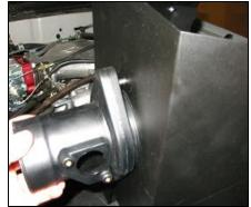
7. Using two supplied <sup>1</sup>/<sub>4</sub>-20 bolts and washers, mount the Airaid filter adaptor to the Airaid Cool Air Dam.
