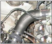
**11.** Connect the Airaid intake tube to the engine by sliding the coupler over the throttle body & adjust the intake tube to insure proper alignment from the throttle body to the air filter adaptor. (*Note: Leave a gap between the tube and the air filter adaptor to allow for engine movement*)
