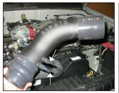
**9.** Install two supplied <sup>1</sup>/4" barbed fittings in AirAid intake tube. (*Note: Install 3/8" fitting in the forward hole and the <sup>1</sup>/4" fitting in the back hole*) Slide hump hose and two #48 hose clamps on large end of intake tube and slide coupler with two #44 hose clamps on small end of tube. (*Note: leave all hose clamps loose for final assembly*)
