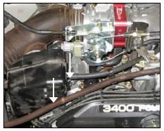
2. Remove factory vacuum lines / hose from the factory air box and intake tube. (*Note: Retain 3/8" vacuum*)
