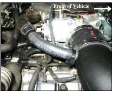
14. Using supplied 5/8" to ½" barbed connector and ½" x 4" hose; connect the factory hose located by the throttle body to the Airaid intake tube. Use two supplied #16 Snapper clamps to secure the hose to the barbed ends.
