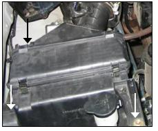
4. With a 12mm socket, remove the three bolts securing the factory air box assembly & remove the factory air box assembly from vehicle.
