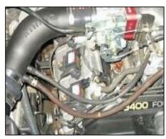
**13.** Connect factory 3/8" vacuum line to nylon fitting on intake tube & connect steel tube on intake manifold to <sup>1</sup>/4" fitting on intake tube with <sup>1</sup>/4" vacuum line provided.
