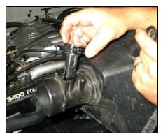
5. Loosen the two screws on the Mass Air Sensor and remove the sensor from the factory air box. <u>Retain sensor for later</u> <u>use.</u>
