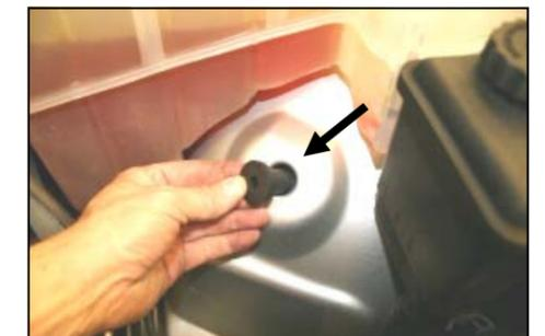
9. Slip the well nut (#21) into the hole in the inner fender.
