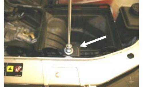
6. With a 10mm socket, remove and save the bolt that holds the factory air filter base to the radiator support. Remove the air filter base from the vehicle.
