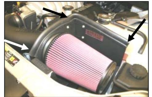
**18.** Install the Airaid Premium Filter (#1), onto the filter adapter inside of the CAD, and tighten the hose clamp. Next install the weather strip (#9) onto the top of the CAD.
