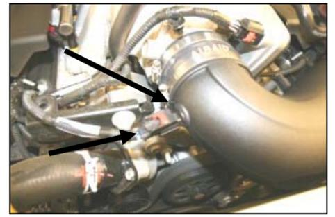
**15.** Install the supplied grommet (#20) into the hole in the Airaid Intake Tube, and then gently push the temperature sensor (*removed in step #4*) thru the grommet until completely seated.
