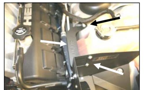
12. Install the rear support bracket (#6) from the CAD to the inner fender using 3 button head bolts (#12), washers (#13), and nuts (#14), and the 10mm factory nut removed in step #11.
