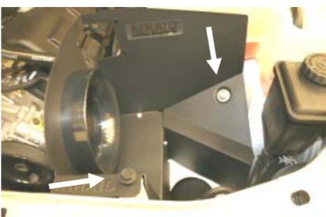
10. Install the assembled Cool Air Dam into the vehicle. Re-install the factory bolt removed in step #6 thru the CAD and into the radiator support. Next install the button head bolt (#10) and washer (#11) thru the CAD and into the well nut. Tighten both bolts.
