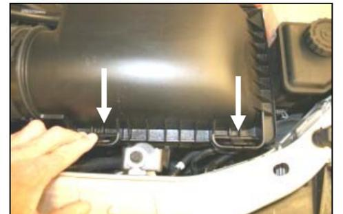
3. Pull both lockdown tabs towards you on the factory airbox lid to remove the lid from the base.
