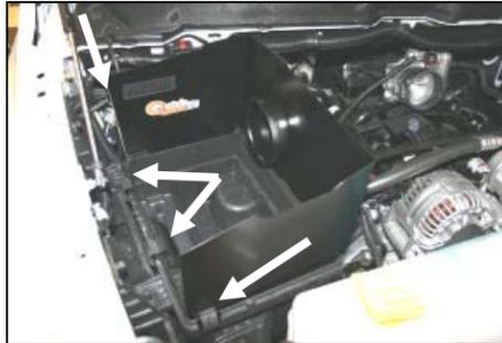
**8.** Install the Cool Air Dam (#2) onto the factory airbox base by sliding the tabs on the base thru the CAD and then adjust the sides to fit. Relatch the 4 clips to hold the CAD securely in place.
