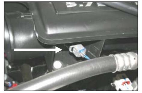
**3.** Squeeze the tab on the connector, and disconnect the intake temperature sensor.
