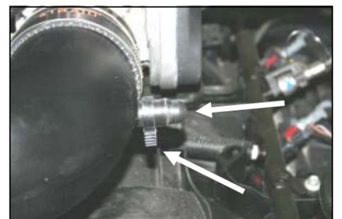
**12.** Install the provided rubber cap (#7) and speed clamp (#10) onto the nipple on the Modular Intake Tube, as shown.
