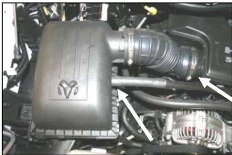
**1. Disconnect the negative battery cable!** Loosen the hose clamp on the resonator. Disconnect the breather hose going into the fac-
