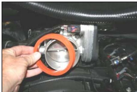
**5.** Remove the factory seal from the throttle body.
