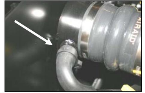
15. Slip the #24 speed clamp (#11) over the factory breather hose and re-connect the factory breather hose to the nipple on the CAD. Squeeze the clamp to retain the hose in place.
