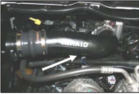
13. (Note: Because production tolerances vary, you may need to remove the tape on the wiring loom and pull out 1 1/2" of wire to the temp sensor, and then re-install the tape. Re-connect the wiring harness to the temperature sensor.)
