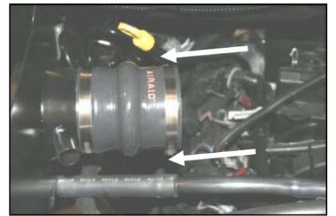
**9.** Install the hump hose (#4) onto the tube on the CAD using two #56 hose clamps (#9). Leave clamps loose.
