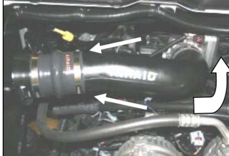
**11.** Install the Modular Intake Tube (#3) into the hump hose first and then into the reducing coupler. Adjust for fit, and then tighten all 4 hose clamps.
