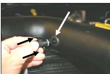
**7.** Install the supplied grommet (#12) into the Modular Intake Tube (#3). Next, carefully slide the factory temperature sensor into the grommet until it touches the tab on the temperature sensor.
