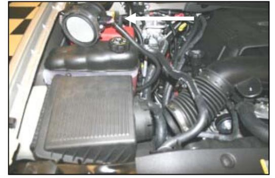
**3.** Without disconnecting the wiring harness, set the Mass Air Flow sensor out of the work area. Next rock the factory air box back and forth, lift it up, and remove it from the hold down grommets. There are no bolts holding it down.
