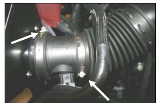
**9.** Re-install the Mass Air Sensor and coupler onto the air filter adapter (#4), as shown and tighten the hose clamp. Next re-connect the factory intake tube to the Mass Air Flow sensor, and tighten the hose clamp.
