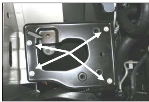
**5.** Remove 4 bolts, and remove the factory air box mounting plate.
