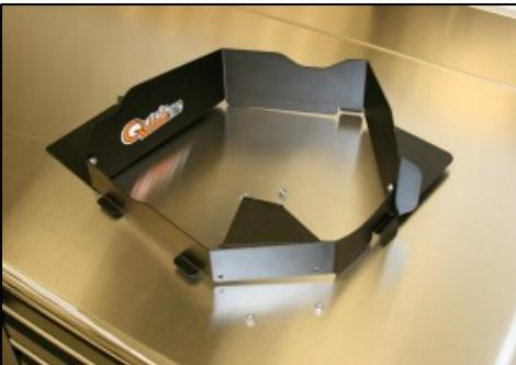
4. Assemble the Airaid Quick Fit Panels together with the four supplied screws, washers, and nuts, as shown.
