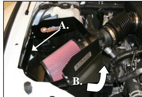
7. **A.)** There are two tabs on the Quick Fit Panel, insert the one closest to the headlight first into the slot on the factory airbox. **B.)** Next, carefully rotate the Quick Fit Panel counterclockwise until the factory clips line up with the tabs on the Quick Fit Panel. Make sure filter tab retains the Airaid Premium Filter. Now lock down the panel with the factory clips.
