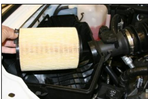
3. Remove the factory air filter from the airbox. Do not remove factory airbox base. The factory base is required to mount the Airaid Quick Fit Panel.
