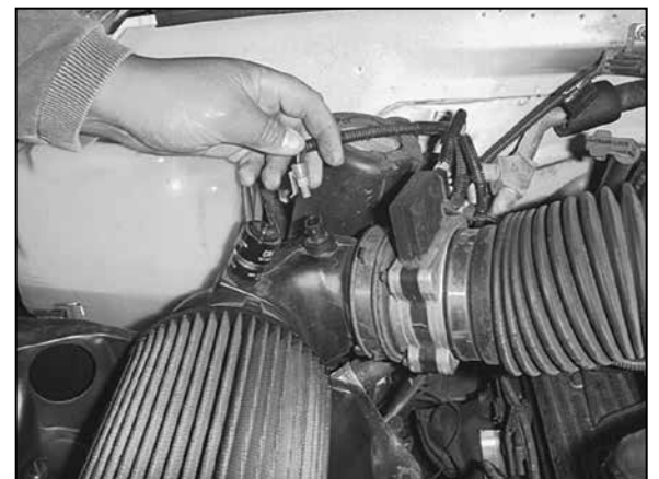
5. Disconnect the air temperature sensor electrical connection.
