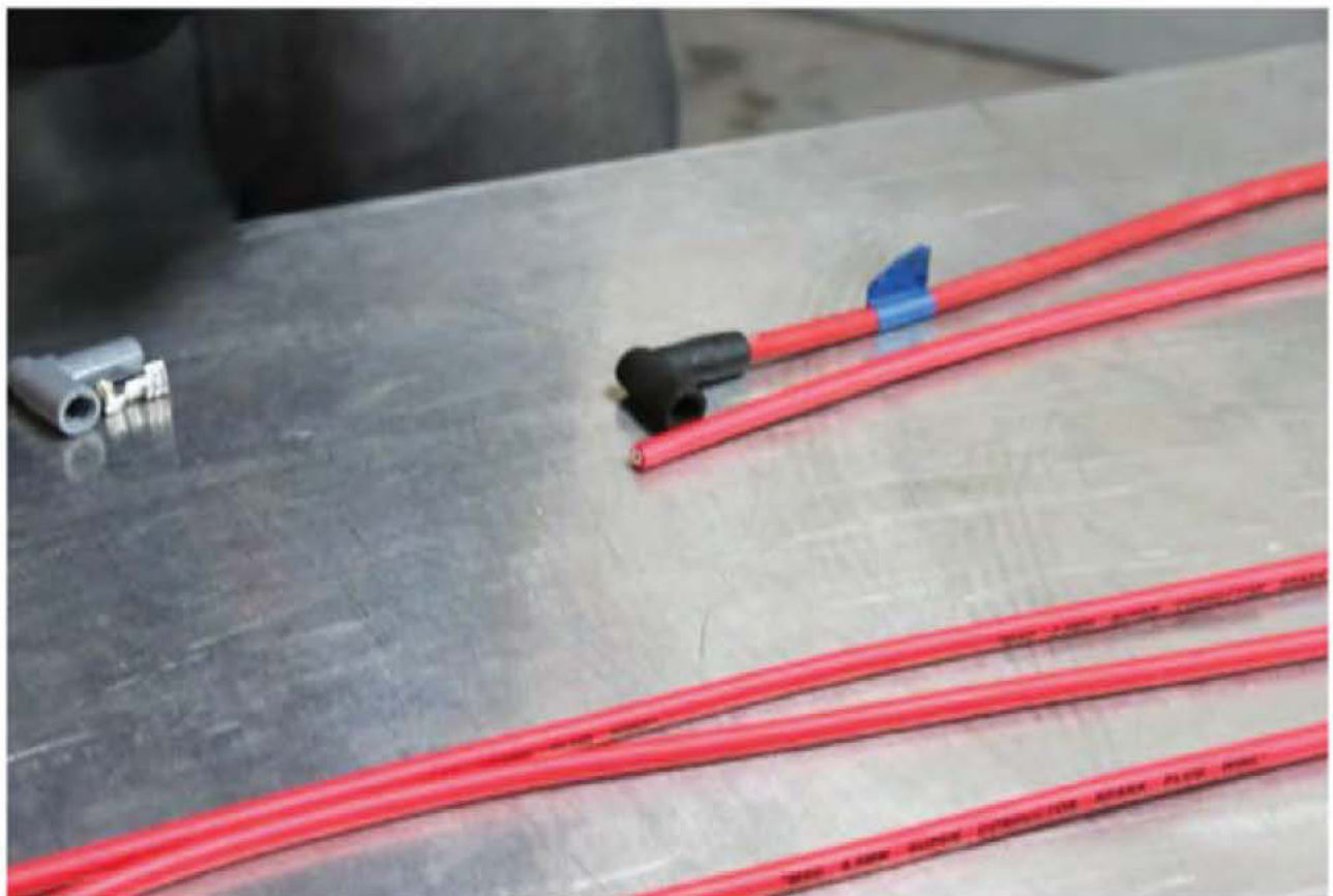
Work with one wire at a time, starting with the longest wire.
