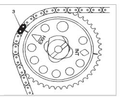
17. Use a 24 mm wrench to rotate the camshaft slightly, until exhaust sprocket aligns with the camshaft.
