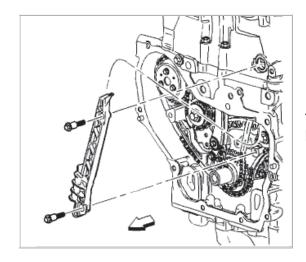
19. Install the fixed timing chain guide. Tighten the fixed timing chain bolts to **15 Nm (133 inch Ibs.)**.
