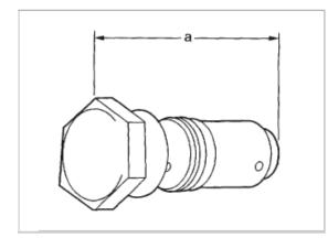
22. Measure the timing chain tensioner assembly from end to end. A new tensioner should be supplied in the fully compressed non-active state. A tensioner in the compressed state will measure 72 mm (2.83 in.) (a) from end to end. A tensioner in the active state will measure 85 mm (3.35 in.) (a) from end to end.
