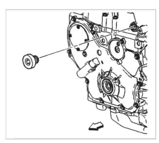
21. Apply sealant. GM P/N 12345382 (Canadian P/N 10953489) to thread and install the timing chain guide bolt access hole plub. Tighten the access hole plug to **90 Nm (66 foot lbs.)**.
