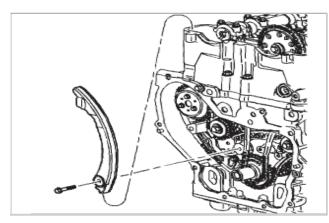
15. Install the timing chain tensioner guide through the opening in the top of the cylinder head. Tighten the timing chain tensioner guide bolt to **10 Nm (89 inch lbs.)**.
