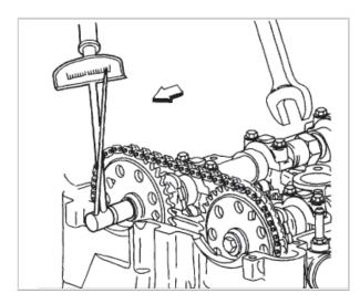
24. The timing chain tensioner is released by compressing it **2 mm (0.079 in.)** which will release the locking mechanism in the ratchet. To release the timing chain tensioner, use a suitable tool with a rubber tip on the end. Feed the tool down through the cam drive chest to rest on the cam chain. Then give a sharp jolt diagonally downwards to release the tensioner. Use a 24 mm wrench to hold the camshaft. Tighten the NEW camshaft bolt to **85 Nm (63 ft. lbs.)** plus 30 degrees.
