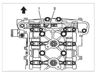
10. Lower the timing chain through the opening in the top of the cylinder head. Carefully ensure that the chain goes around both sides of the cylinder block bosses. (1,2)
