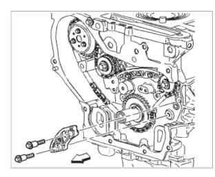
1. Install the upper balance shaft chain guide. Tighten the upper balance shaft chain guide bolts to **15 Nm (133 inch lbs.)**.
