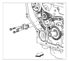
5. Install the timing chain tensioner.
